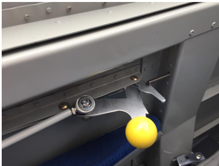
FIGURE 2: CANOPY LATCH PRE ENGAGEMENT OF CANOPY SWITCH
