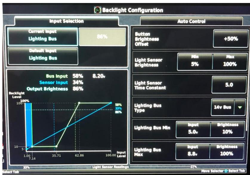
**FIGURE 4: G3X Backlight Configuration**
